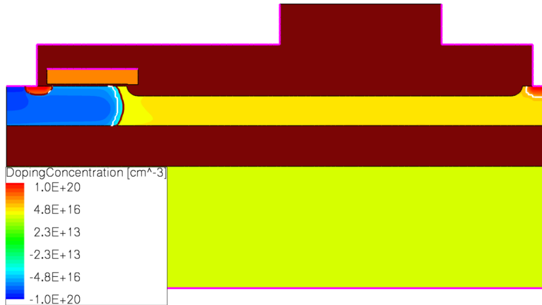
Figure 60: Simulated Doping Concentration of 150 V SOI Resurf LDMOS Without Buffer
