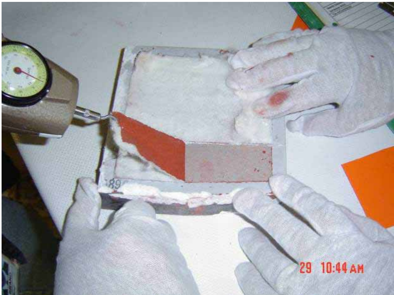
Figure 26 - SIP Peel Test Being Performed on Subnominal Bond Tile
