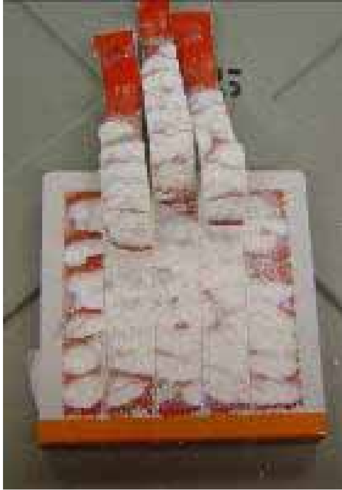
Figure 43 - SIP Peel Test with 0.78g of RTV Applied
