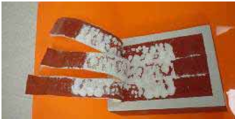
Figure 39 - SIP Peel Test without Silane Average Peel 6 lb/in
