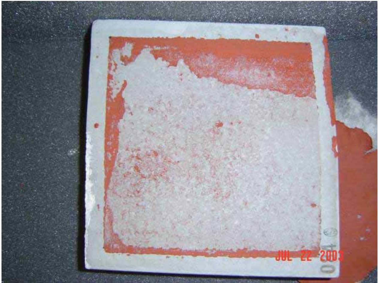
Figure 22 - OV-105 Subnominal Bond Condition
