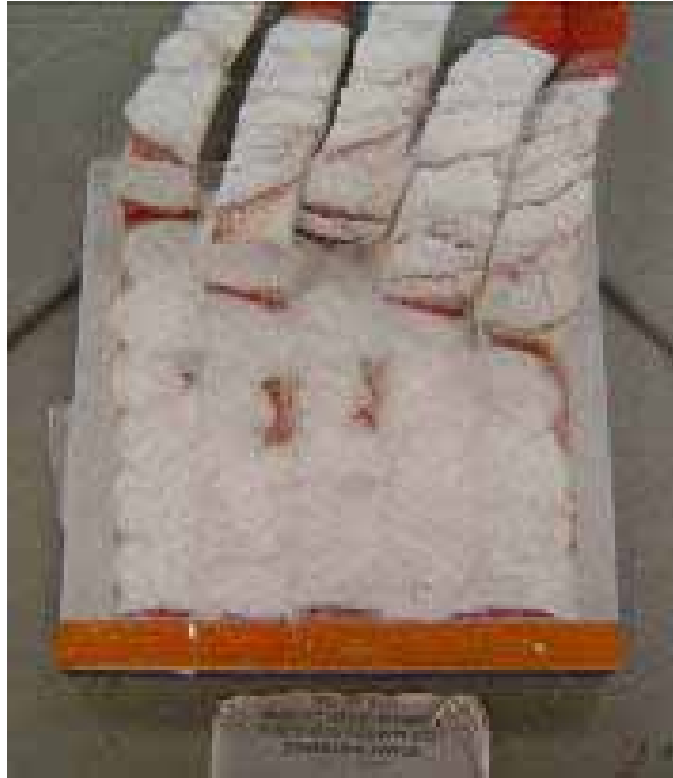
Figure 42 - SIP Peel Test with 3.61g of RTV Applied
