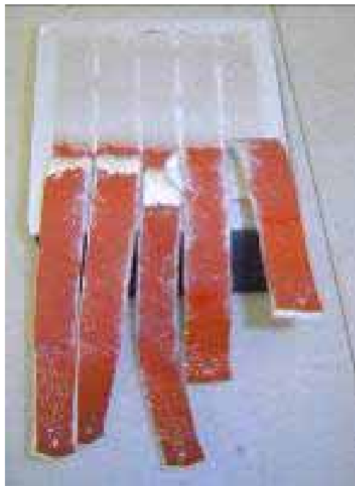
Figure 44 - SIP Peel Test with Krylon 1201 Spray Starch
