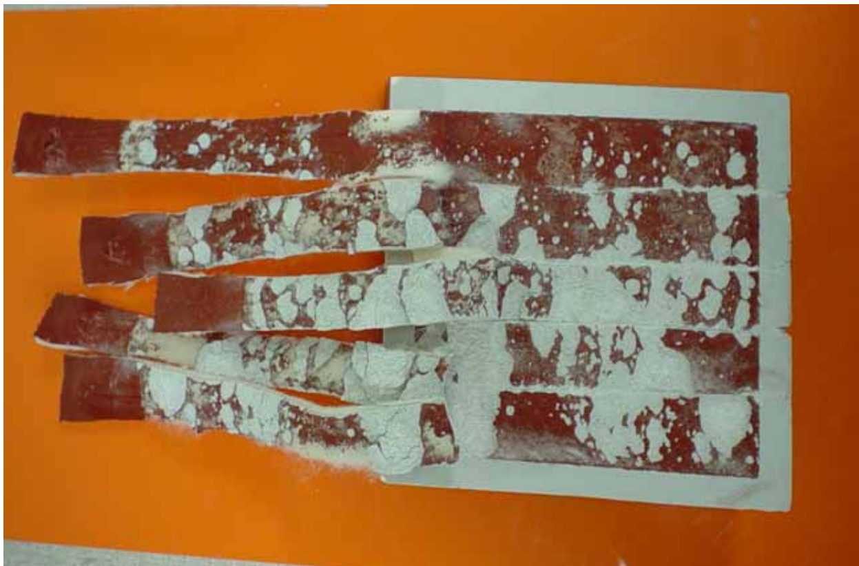
Figure 38 - Peel without Waterproofing; Average Peel 13.5 lb/in
