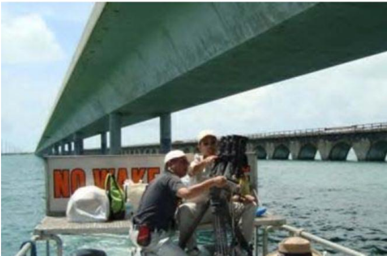
Figure 11: Bridge Inspection using High Definition Video Camera
