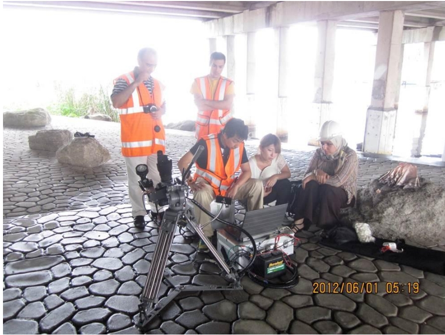
Figure 12: Bridge Inspection using Motion-Controlled Digital Camera
