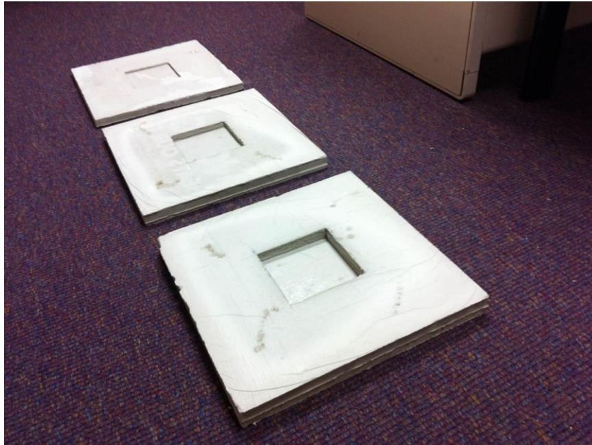
Figure 39: Concrete Test Pieces (Different Volume of Delamination)
