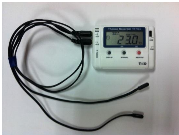
Figure 32: Temperature Measurement Sensor
