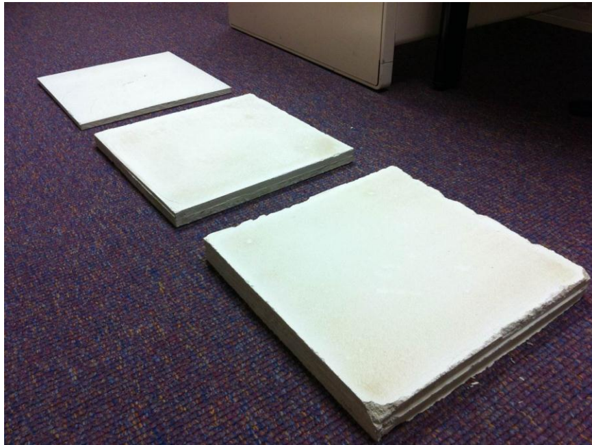
Figure 38: Concrete Test Pieces (Different Thickness)
