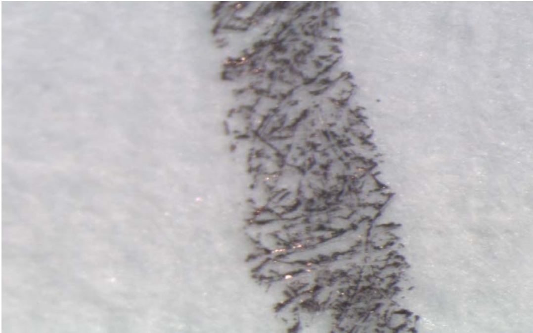
Figure 1: Black ballpoint ink on plain white copy paper, enlarged to show detail, 30-minute drying time
