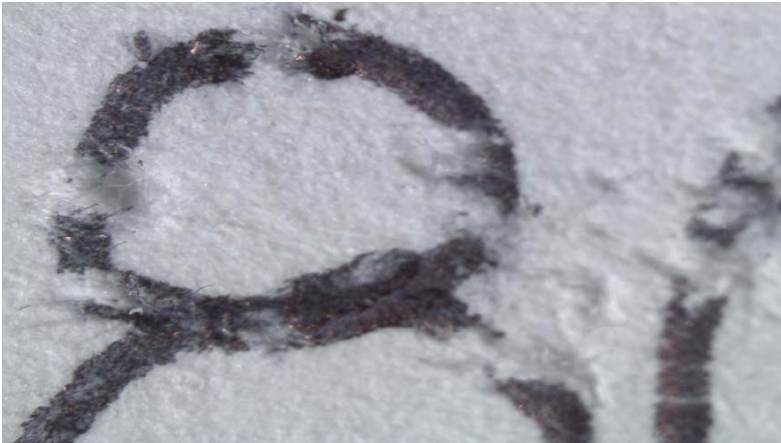
Figure 22: After sampling, showing the sampling of overlapping ink from pen 3 and pen 5
