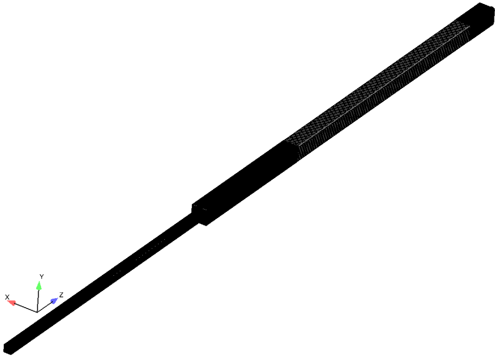
Figure 28: Entire mesh for head end only model (flow in z direction)
