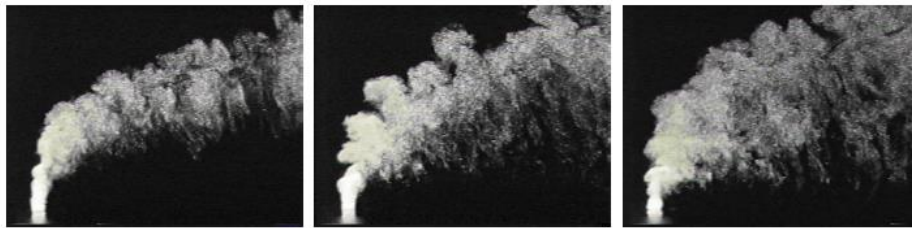
Figure 8: Flow visualization from experiments of a jet injected into a steady (left) and unsteady (center, right) cross flow (Blossey, 2002)
