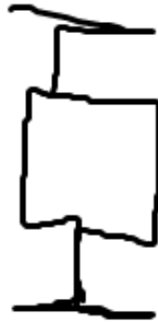
Figure 22 – Example of duplicated points and self-intersections
