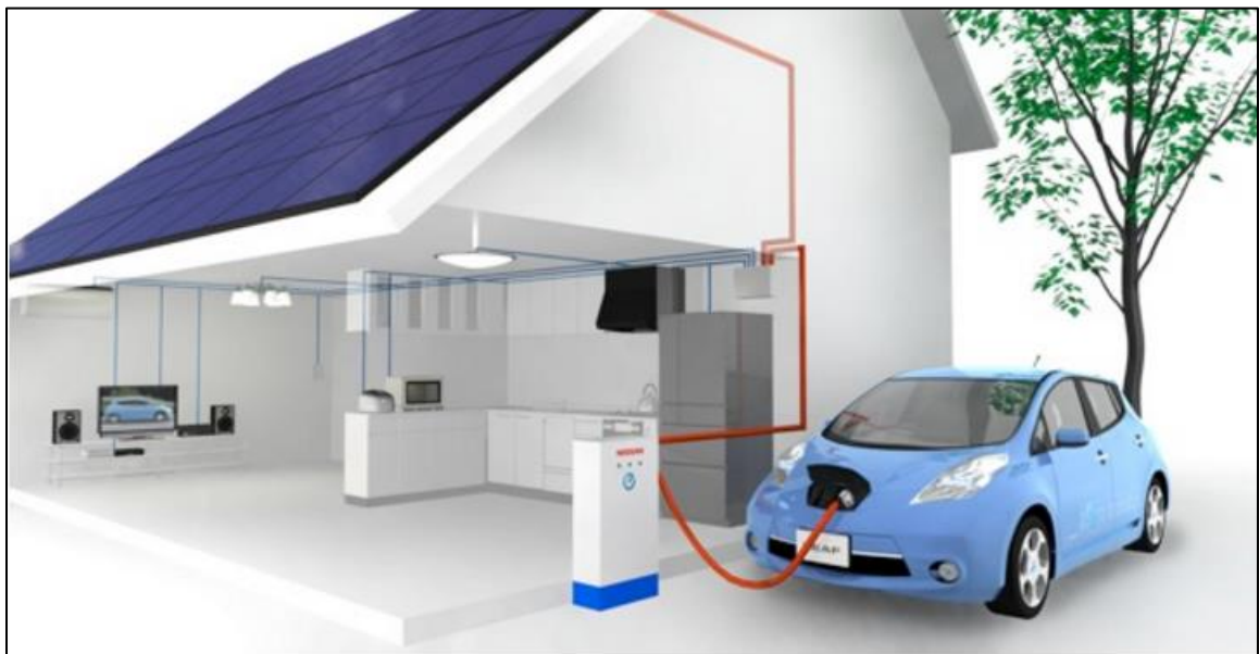
Figure 7. Power transmission from EV to building [72]
