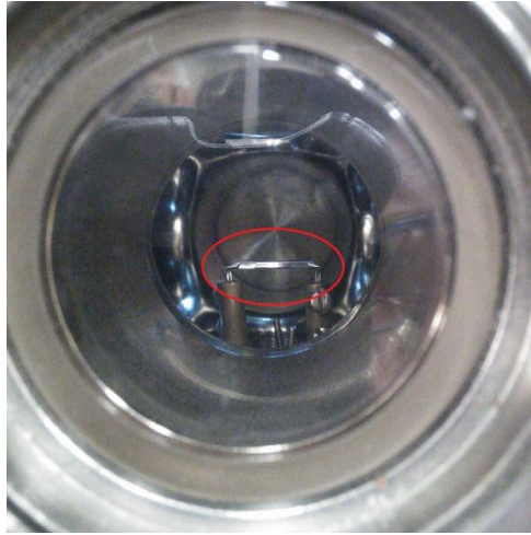
Figure 6.3: An alkali metal dispenser in an UHV chamber. The electrodes extend outside of the chamber to pass current through the dispenser.
