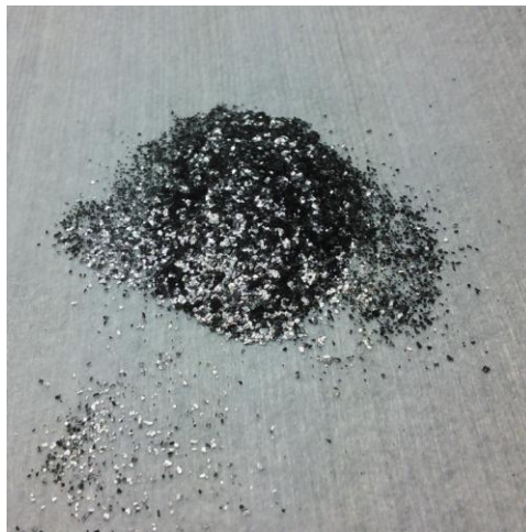
Figure 1.1: An image of graphite flakes. Graphite is made of a stack of graphene. Carbon nanotubes and C_{60} are conceptually constructed from graphene by forming a tubular shape and buckyball, respectively.
