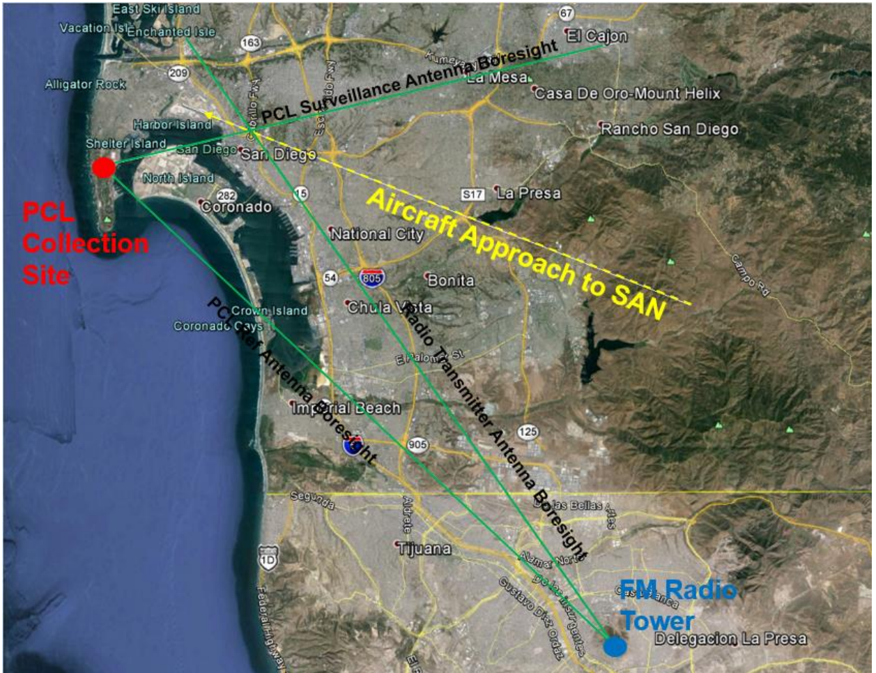
Figure 3.6: PCL experiment geometry. Map data taken from 2016 INEGI, SIO, NOAA, U.S. Navy, NGA, GEBCO, 2016 Google, USGS.
