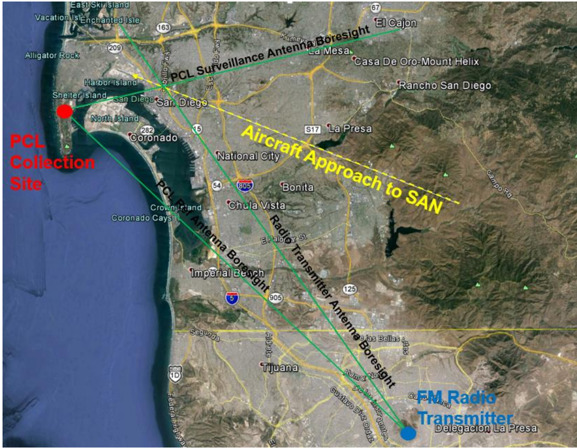
Figure 6.2: Multi-channel PCL experiment geometry. Map data taken from 2016 INEGI, SIO, NOAA, U.S. Navy, NGA, GEBCO, 2016 Google, USGS.
