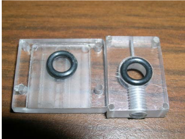
Figure 60. O-rings are in black, the rectangles are the polycarbonate package components, bottom threaded leur fitting
