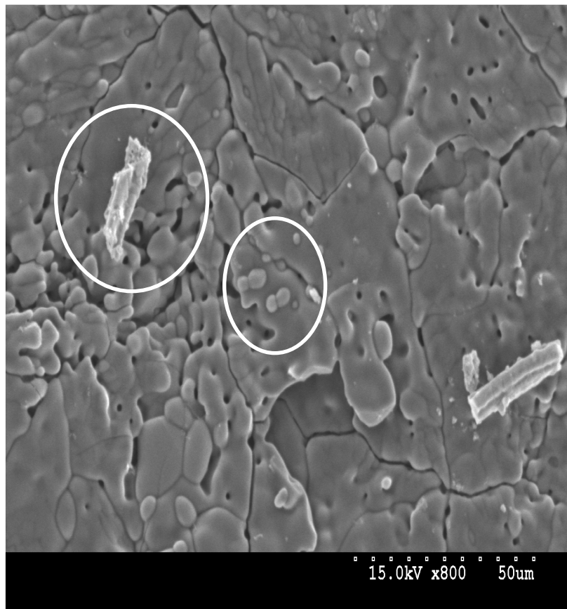
Figure 21. SEM images of sintered \text{Al}_2\text{O}_3 - \text{Al}_2\text{TiO}_5 - \text{TiO}_2 nanocomposite pellets soaked in SBF for 14 days shows highlighted regions with crystals of apatite in various shapes and sizes.
