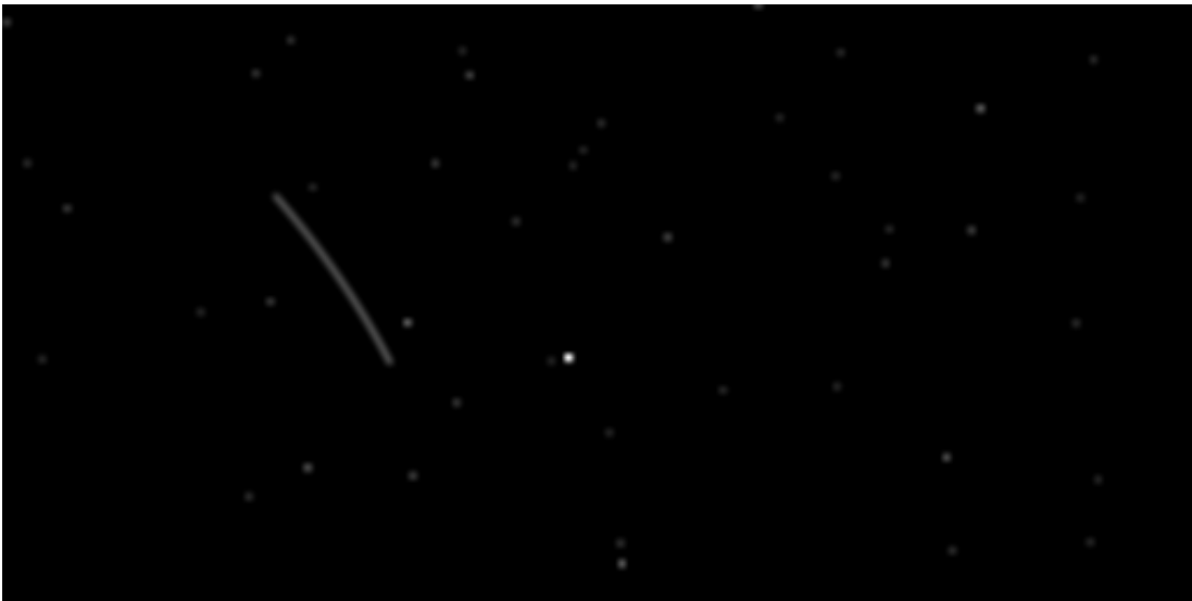
Figure 2.8: Complete full-frame star camera image with pronounced RSO streak.
