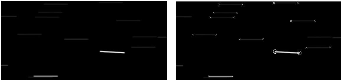
Figure 4.6: Sample RSO detection during spacecraft slew with constant angular rate.
