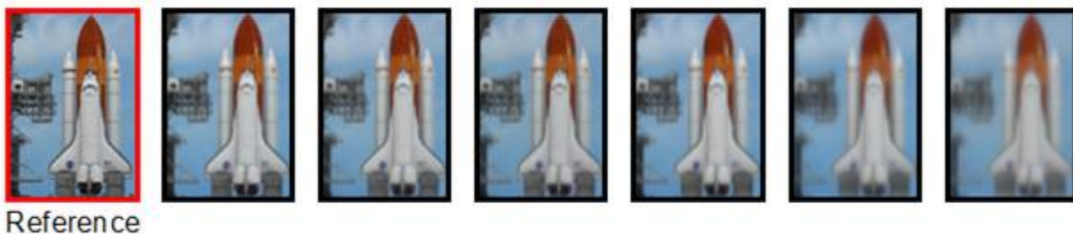
Figure 37. Just Noticeable Differences are determined from a sequence of paired comparisons. The reference image (outlined in red) is paired with each of the remaining 6 test images, creating six pairs of images.
