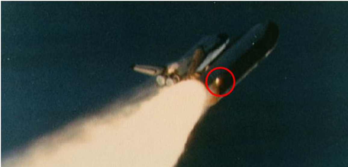
Figure 4. Launch imagery of the Space Shuttle Challenger shortly before exploding, showing evidence of unexpected flame (circled) emitted from the side of one of the solid rocket boosters.
