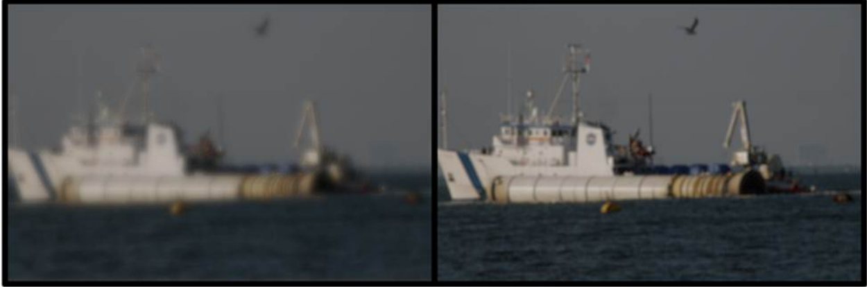
Figure 19. Two images degraded with equal RMS wavefront error ( 0.4\lambda ) when the aberration is balanced spherical aberration (left) and balanced astigmatism (right).
