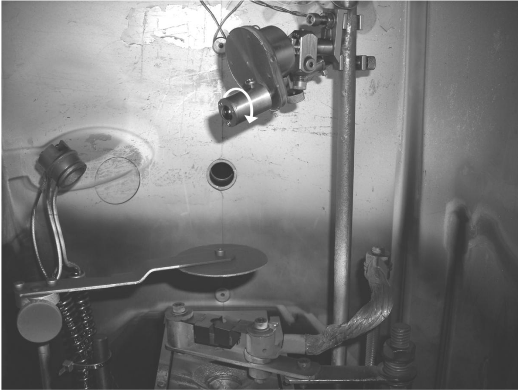
Figure 11: Rotating device inside the evaporation chamber. The hemispherical lens is 14 cm above the thermal source and rotated in a direction indicated by the white arrow.
