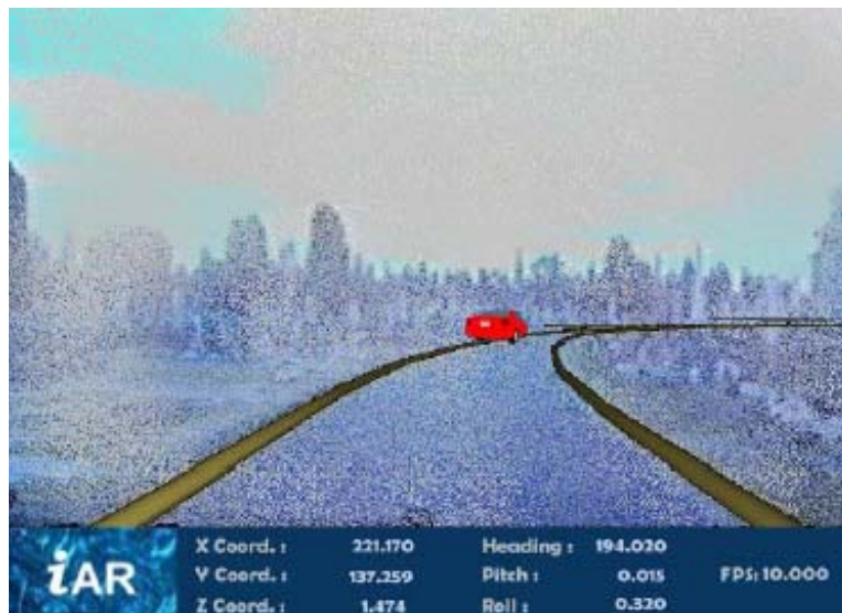
Figure 2-22: The AR system shows road edges and a near vehicle as displayed to the driver (Scott-Young et al. 2003).
