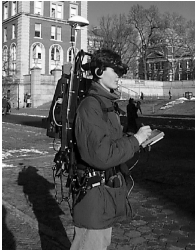
Figure 2-2: Mobile optic AR system with HMD and a hand-held display (Feiner et al. 1997).
