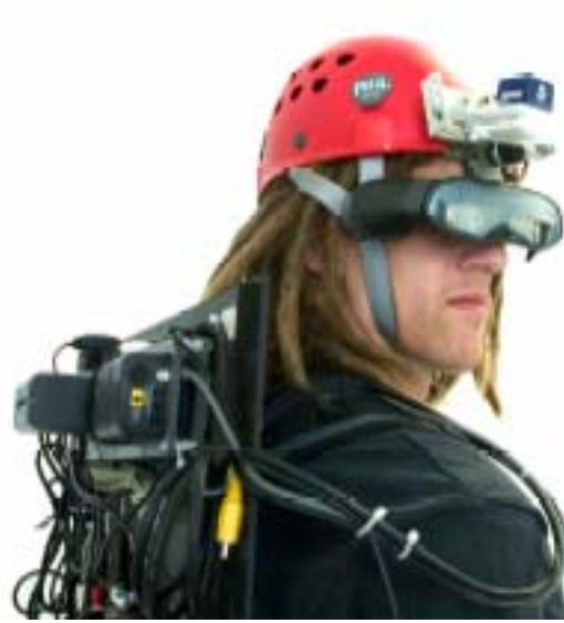
Figure 2-4: Mobile video AR system with HMD (Wagner et al. 2005)
