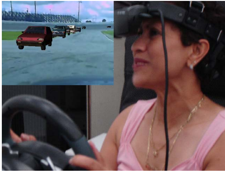
Figure 7-8: Left turning maneuver at two-way stop-controlled intersection experiment using the OARSim system.
