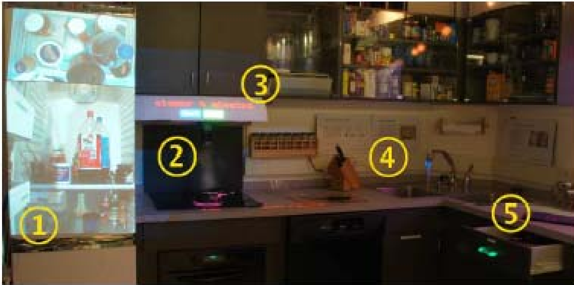
Figure 2-24: Augmented reality kitchen, information is projected on the refrigerator (1), the range hood (2), the cabinet (3), the faucet (4), and the drawer (5) (Bonanni et al. 2005).
