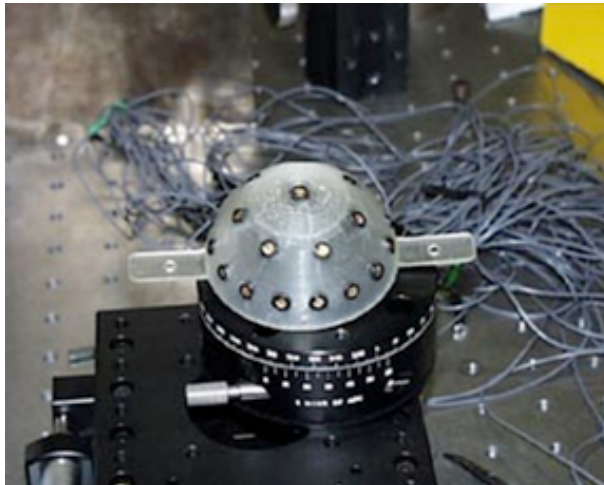
Figure 6.11: A Semi-spherical Head Tracking Probe
