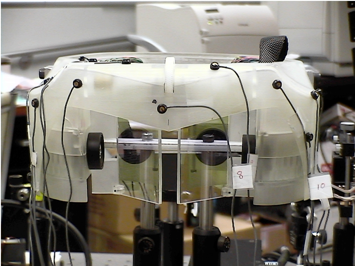
Figure 6.15: Realization of a Conformally Mapped Tracking Probe
