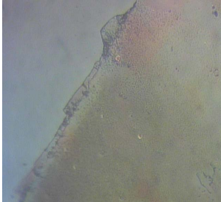
Figure 74 Nanotube/SnO 2 thin film under 500X microscope
