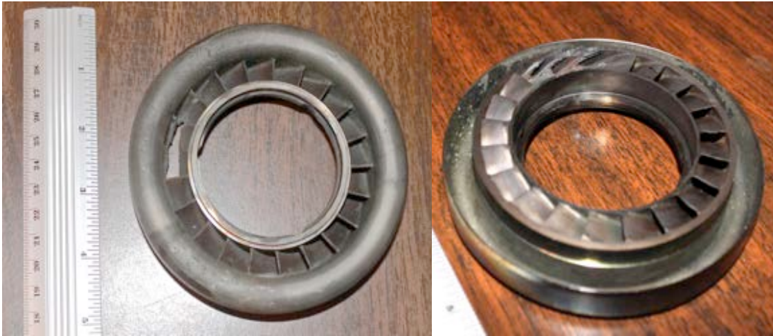
Figure 18 – Turbine stator damage
