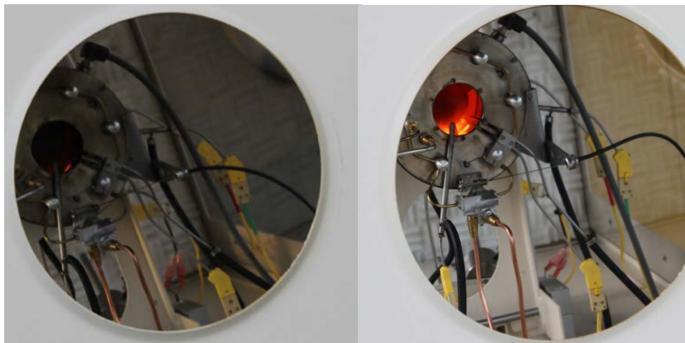
Figure 20 – Localized overheated zone after repair (left) and before repair (right)
