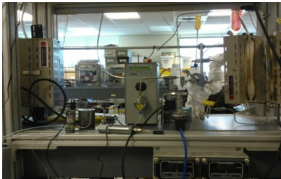
Figure 3 – Photograph of fuel thermal stability rig
