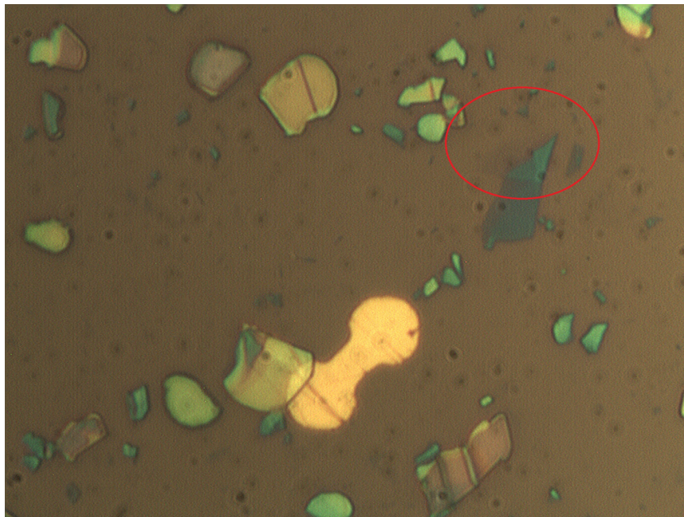
Figure 3.2: Optical Image of Exfoliated hBN Flake. Optical micrograph showing an exfoliated and bulk hBN flake. Thicker hBN crystals are yellow in color, then change from green, to blue as the number of layers decreases. The thin region used to create a device is circled in red.
