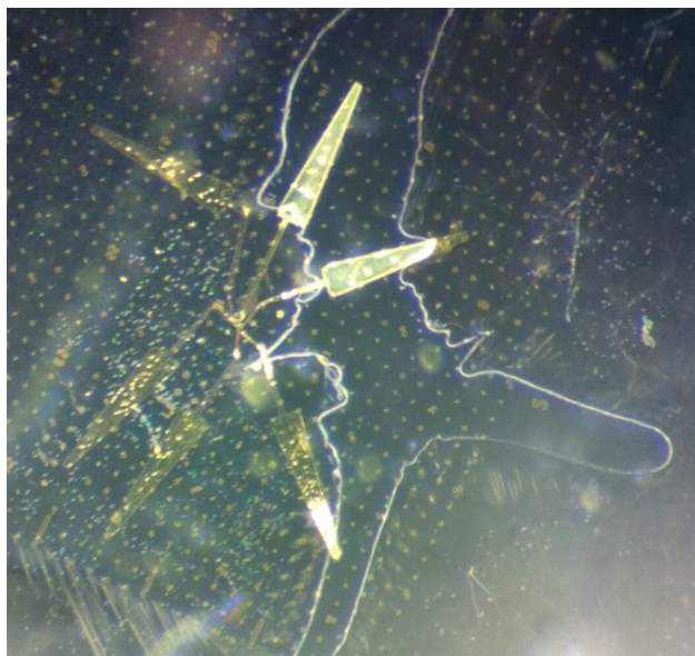
Figure 1.16: Electrodes transferred to Transparent Substrate. Partially transferred electrode pattern at 100x magnification. The brighter gold has been transferred to the transparent substrate correctly.
