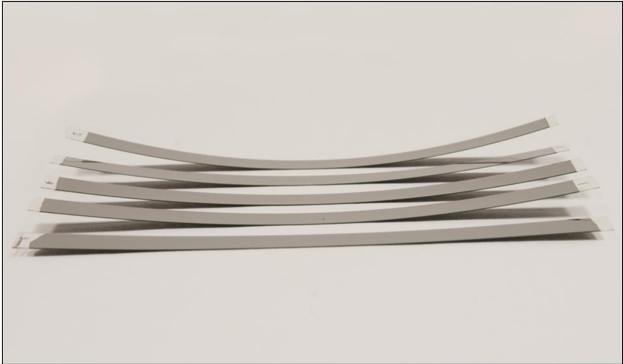
Figure 4.38: Bending of glass strips with molybdenum films deposited at various processing conditions
