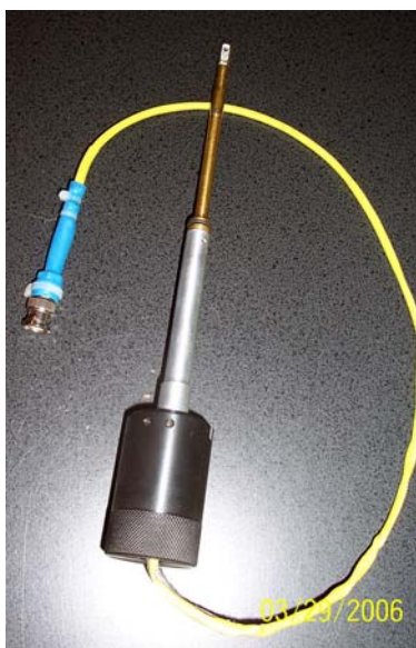
Figure 15. Specimen holder for EBIC measurements which allows electrical contact between specimen and microscope electronics..
