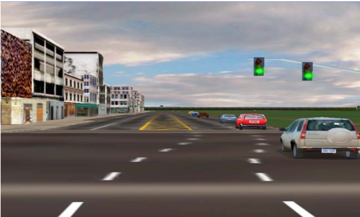
Figure 5-18: Approaching intersection with lane misalignment and striping present
