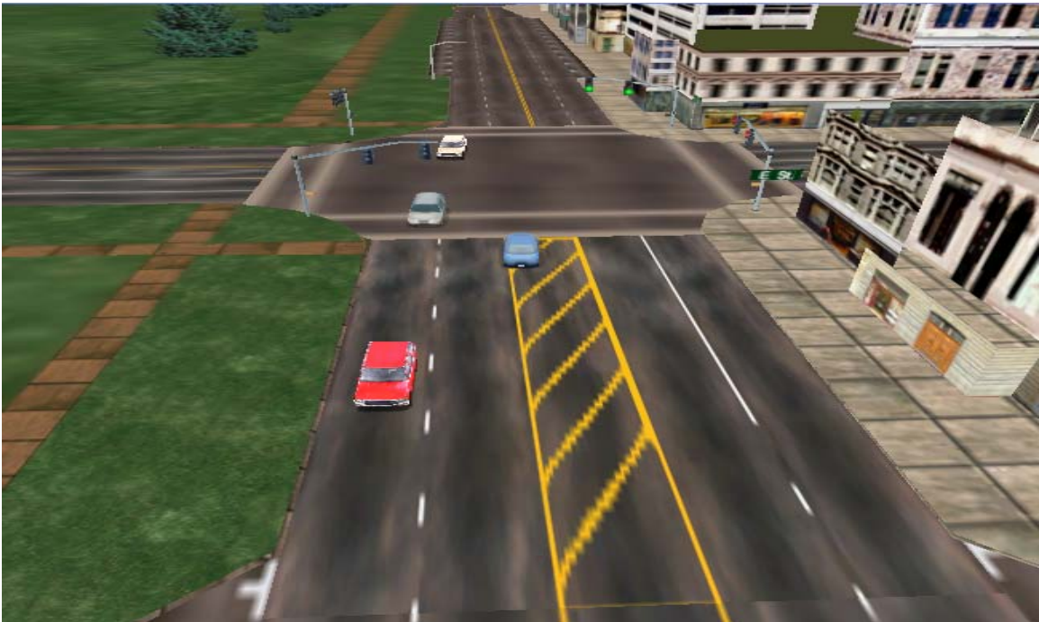
Figure 5-16: Overhead view of simulator vehicle exiting intersection with lane misalignment and no striping
