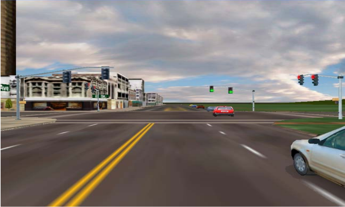
Figure 5-13: View through the windshield of simulator vehicle approaching the intersection with lane misalignment and no striping
