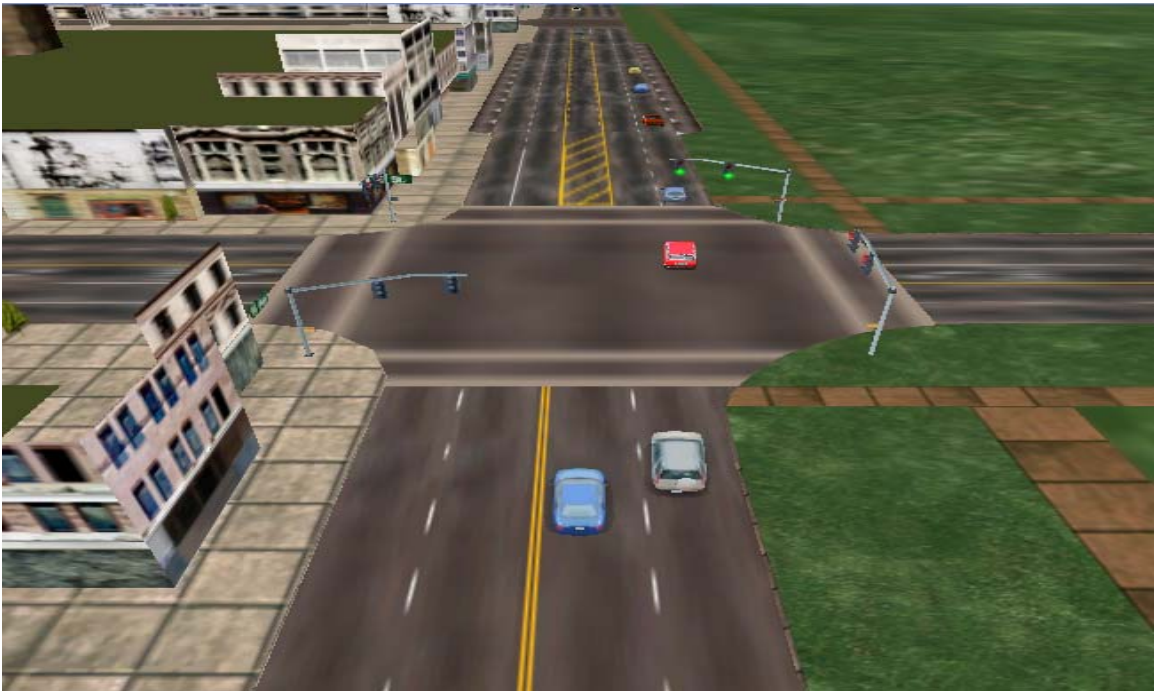
Figure 5-14: Overhead view of simulator vehicle approaching the intersection with lane misalignment and no striping
