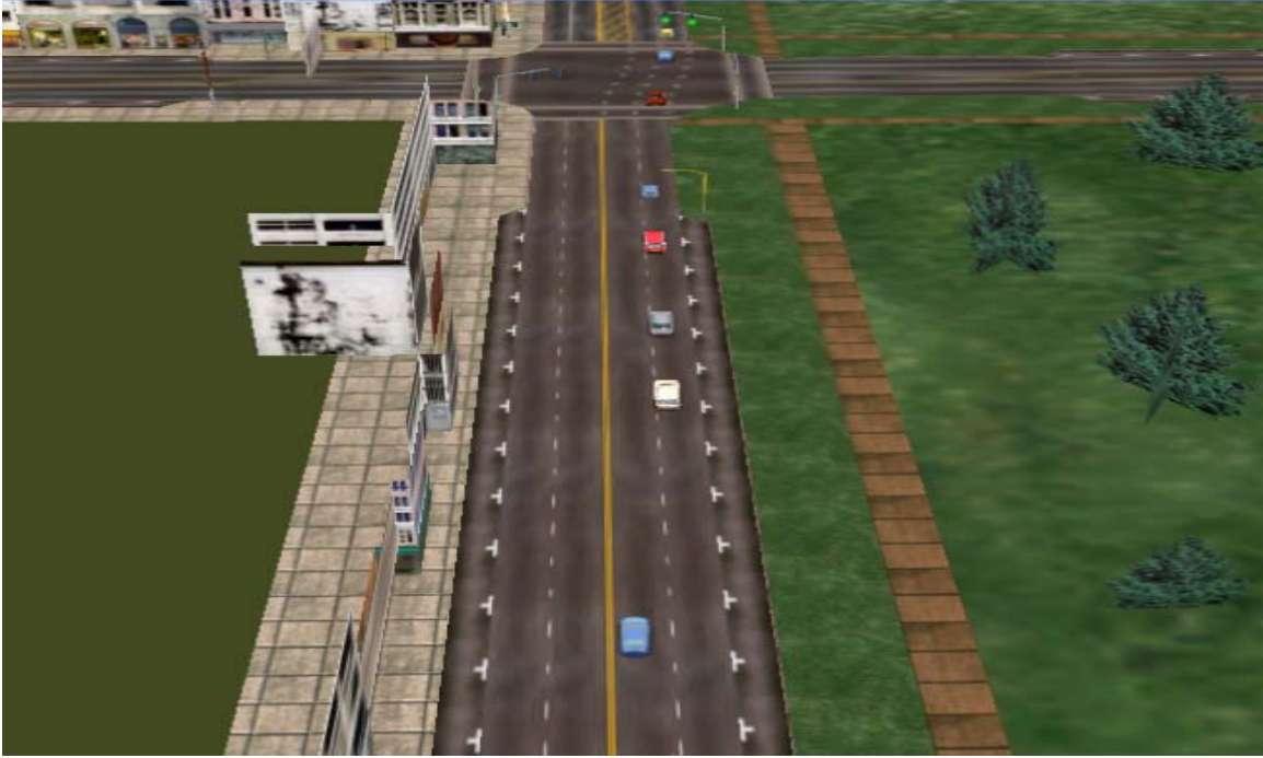
Figure 5-17: Overhead view of simulator vehicle upstream from intersection with lane misalignment and striping present
