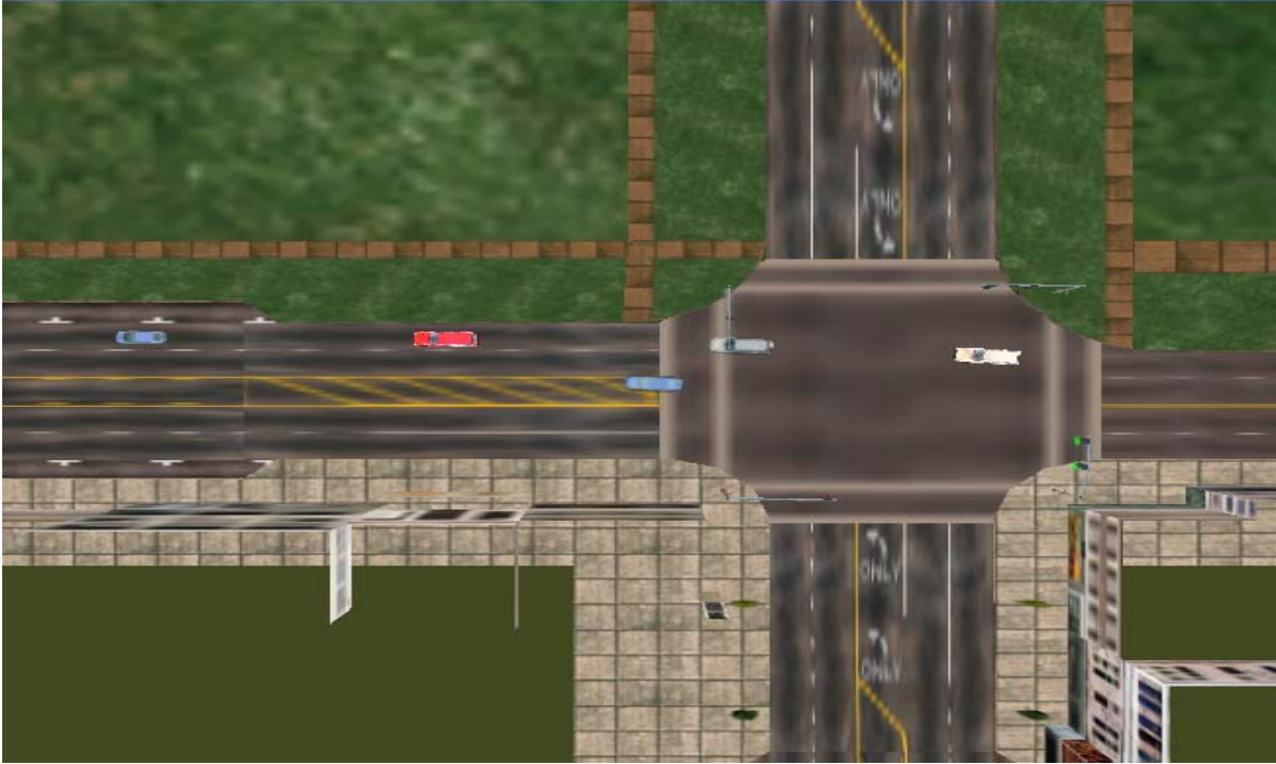
Figure 5-15: Overhead view of simulator vehicle in intersection with lane misalignment and no striping
