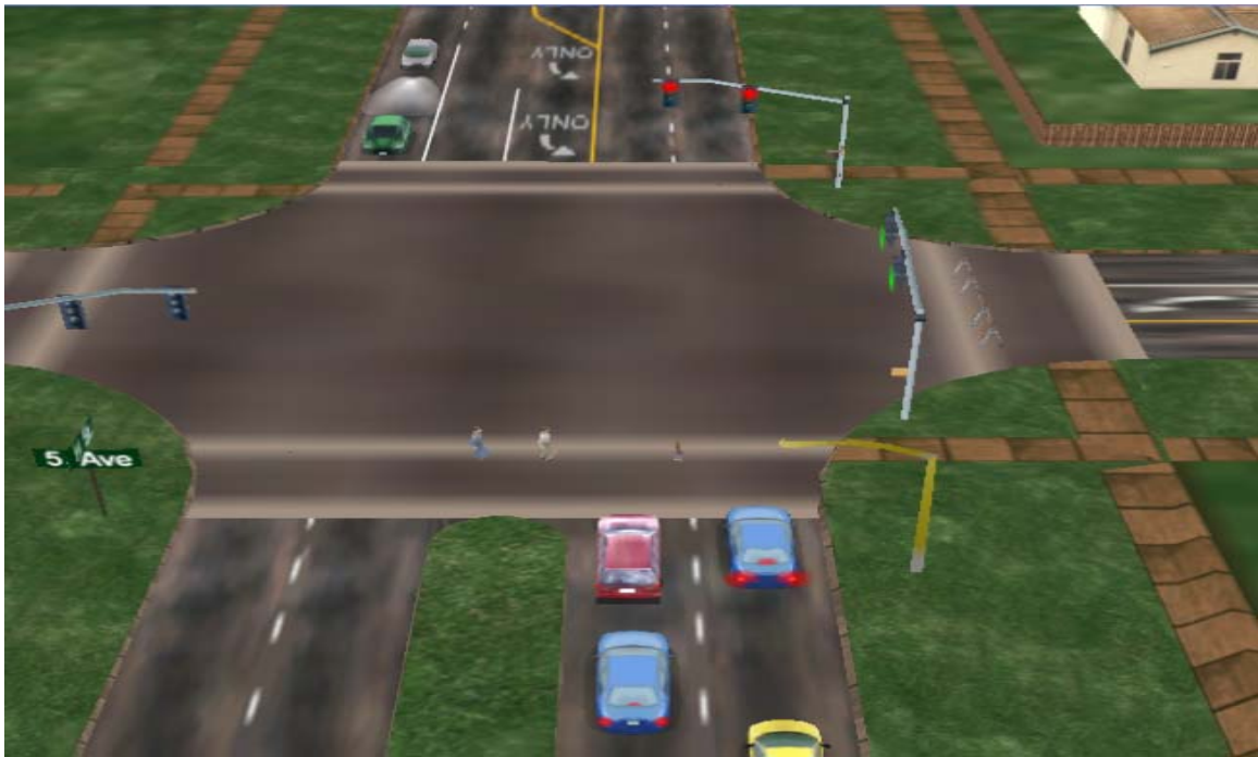
Figure 5-20: Simulator vehicle stopped at red light in a joint left and through lane
