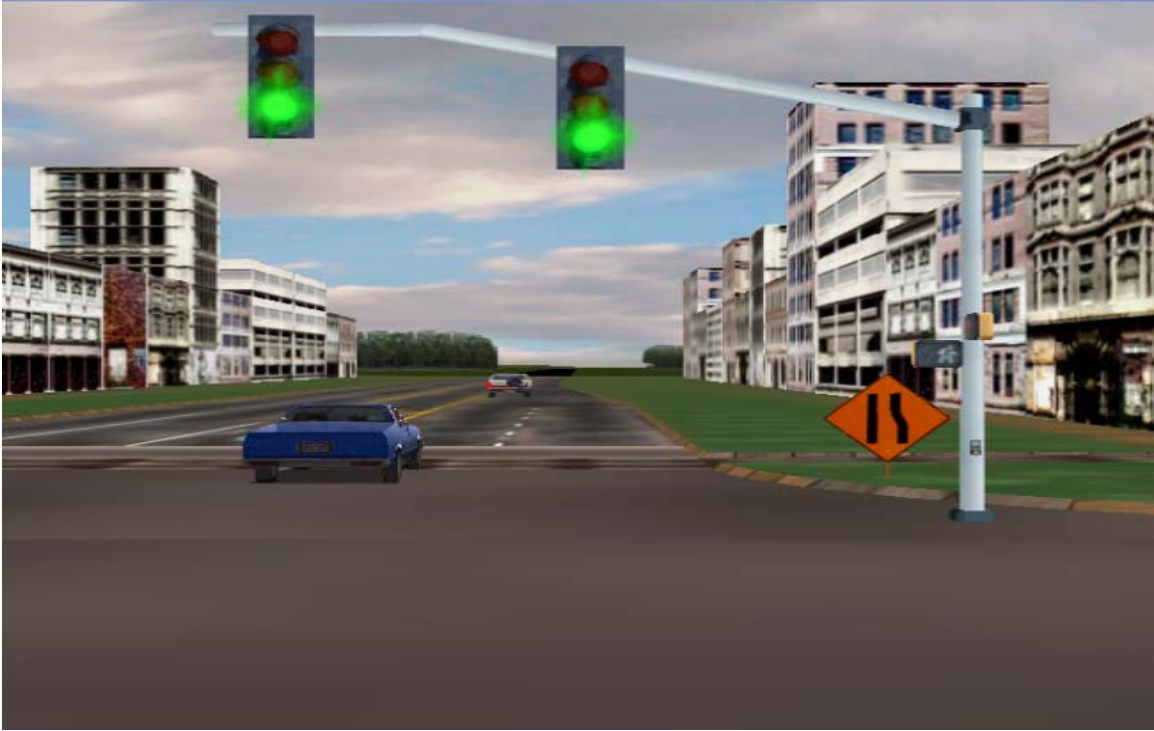
Figure 5-5: Approaching intersection with short dropped lane
