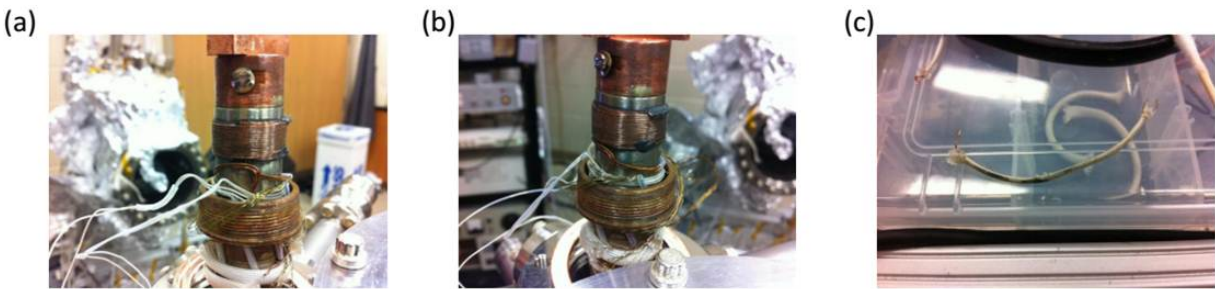
Figure 2.19: : (a), (b) Pictures showing heater with black color residue from outgassing of the stycast, and (c) Picture showing black color contamination on the wire selves used for tying the wiring on the Helit-ran.
