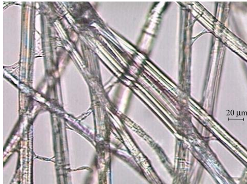
Figure 3.4. Synthetic cotton-like cylindrical fibers having in average a diameter of 20\mu m .
