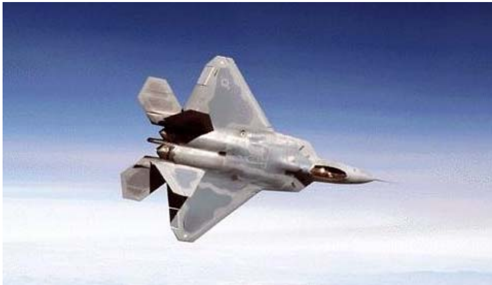
Figure 2: The Lockheed F-22, using composites for at least a third of its structure
