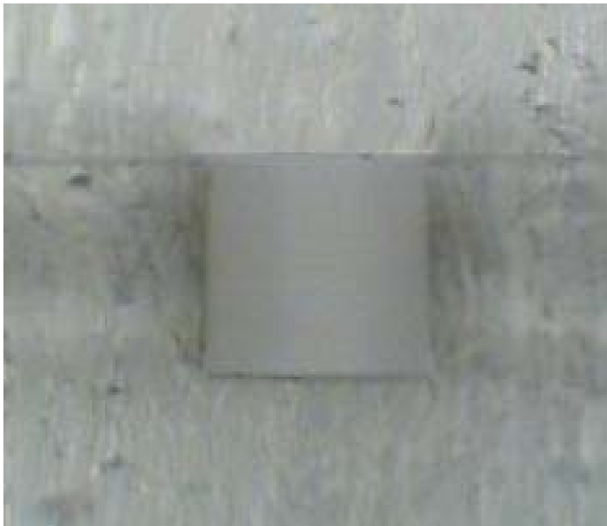
Figure 21: Cross-sectional slice of a sample microchannel.
