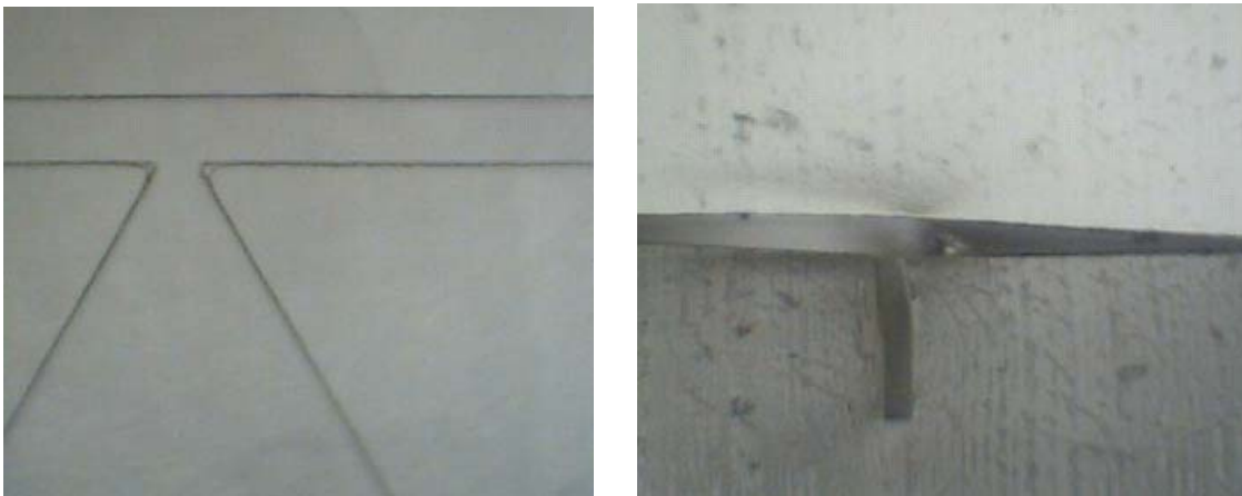
Figure 35: Channel leakage due to PDMS slab separation.
