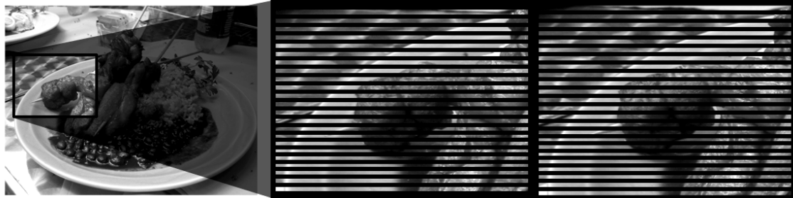
Figure 5: A close up look at an NTSC image (left) reveals odd (middle) and even (right) interlaced frames (Hutchens, 2007e)
