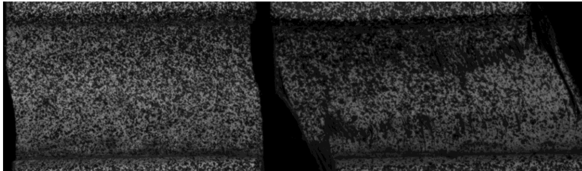
Figure 12: Comparison of last test step in shear tests between displacement control (left) and force control (right) shear tests
