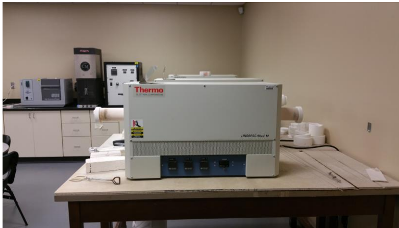
Figure 16 Lindberg Blue M Three-Zone tube furnace used in heat treatments
