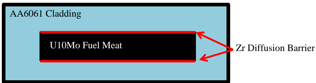
Figure 3 Schematic diagram of U10Mo-Zr-AA6061 monolithic fuel plate
