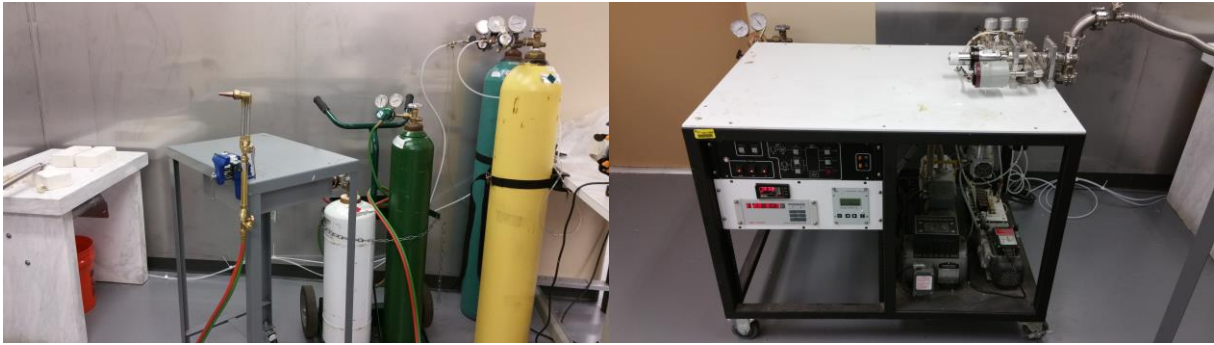
Figure 15 Encapsulation system: acetylene torch(left) and vacuum system(right).
