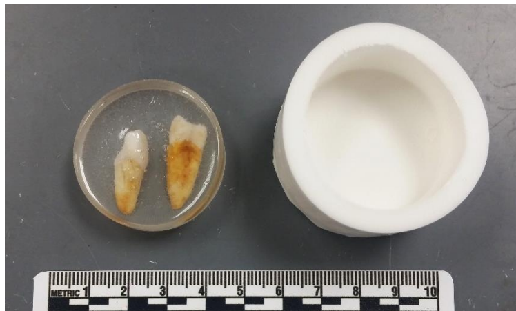
Figure 4: Two test teeth embedded in hardened epoxy resin (left) and the silicone mold previously containing resin with teeth (right).
