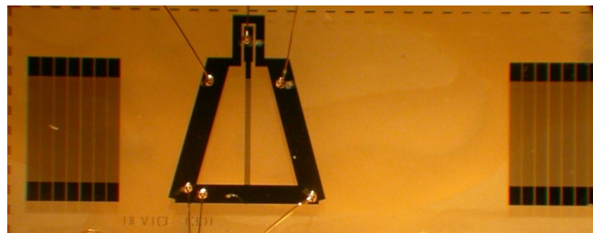
Figure 8-2. Dual-sided OFC SAW Device on \text{LiNbO}_3
