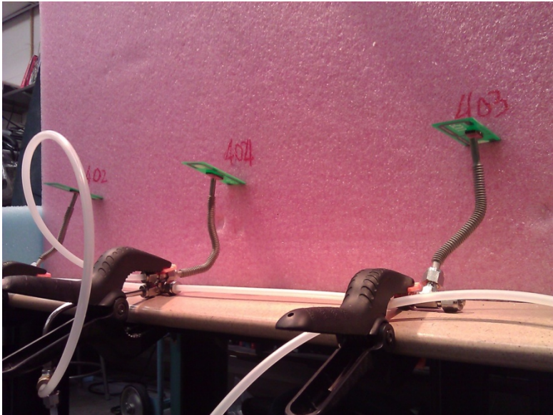
Figure 7-10. This is a picture of the 3-way splitter and the gas flow to the three sensors.
