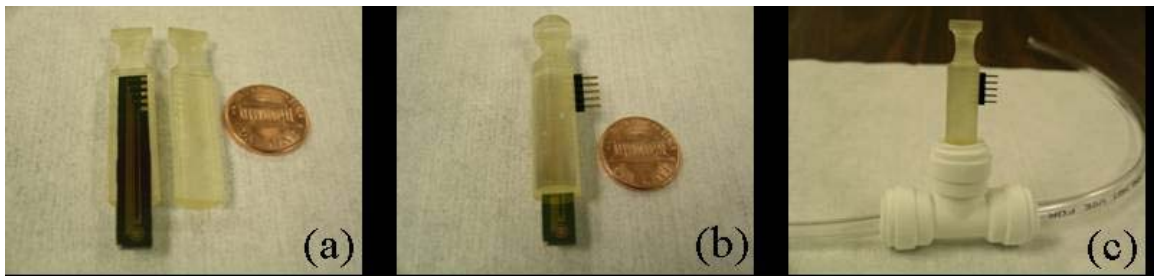
Figure 5.4: Assembled view of the plug-in type package with micromachined sensor.
