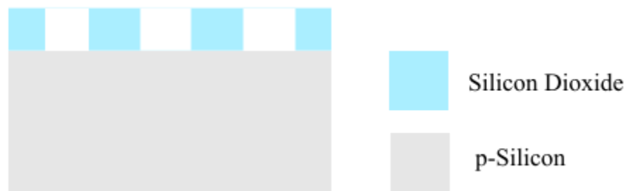
Figure 4.3: Substrate Cross Section after First Mask And Oxide Etch
