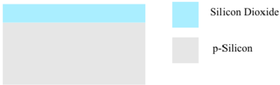
Figure 4.1: Silicon Substrate Cross Section after Gate Oxidation
