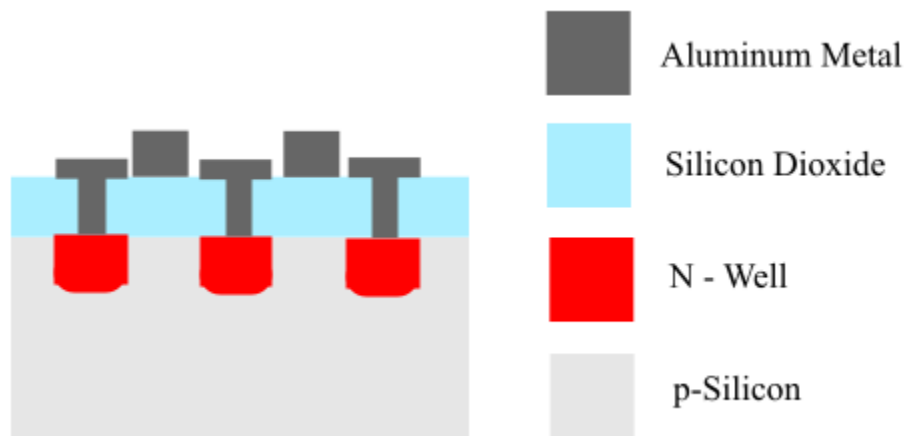
Figure 4.16: Cross Section of Aluminum Gate Contact MOSFET
