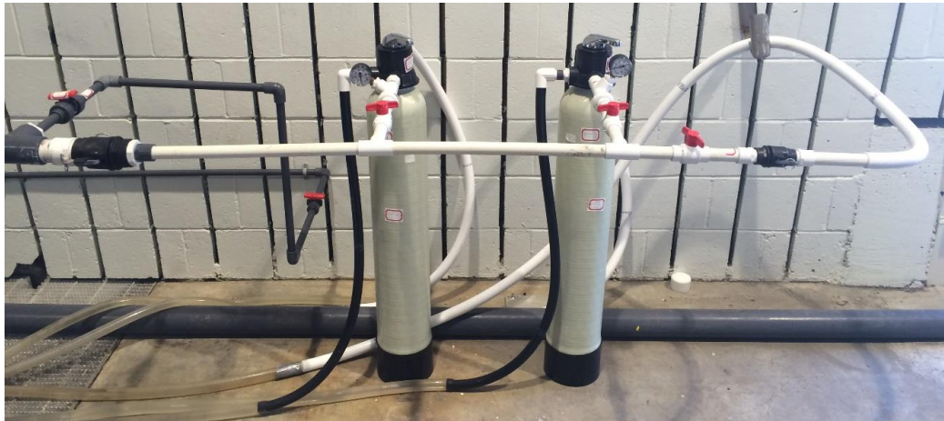
Figure 4-3: Bench-Scale Parallel Sand Filtration Unit
