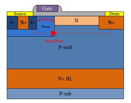
Figure 1.1 A typical power MOSFET structure with the inherent body diode
