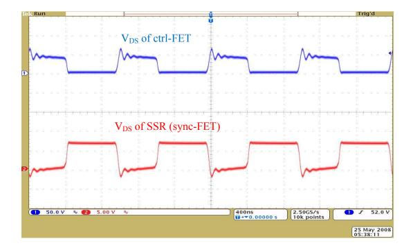
Figure 3.6 Operating waveforms at 1MHz
