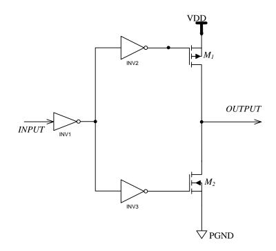
Figure 4.9 Driver for MOSFET switches in high-side driver
