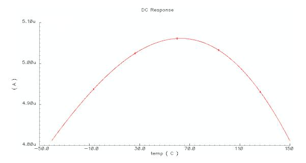
Figure 2.8 Current source temperature dependence (typ.l)
