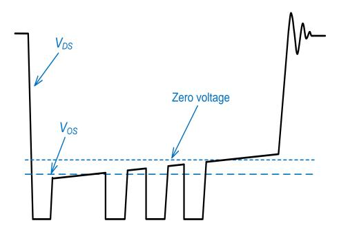
Figure 2.11  $V_{DS}$  waveform with oscillation for  $V_{OS} < 0$  under light load
