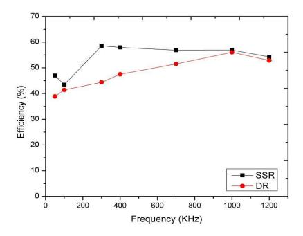
Figure 3.10 Measured efficiency vs. switching frequency
