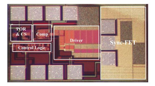
Figure 2.20 Photo of the self-synchronized rectifier chip
