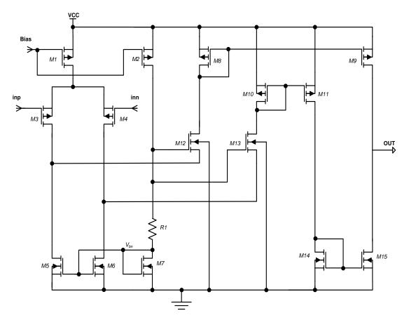
Figure 2.12 Schematic of the voltage comparator
