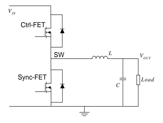
Figure 1.2 A typical synchronous buck converter
