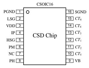
Figure 4.12 CSD chip pinouts
