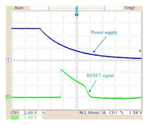
Figure 2.22 UVLO at Power-down transient
