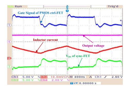
Figure 2.28 Measured switching waveforms of the buck converter at 1MHz
