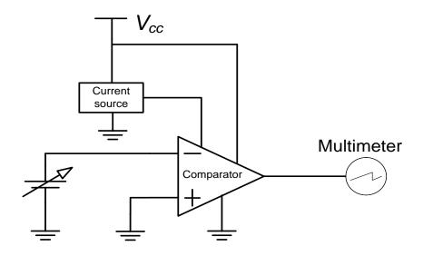
Figure 2.24 Comparator offset voltage testing setup
