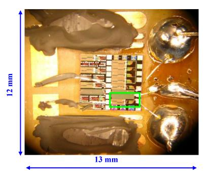
Figure 5.6 The buck PSiP after ferrite epoxy coating
