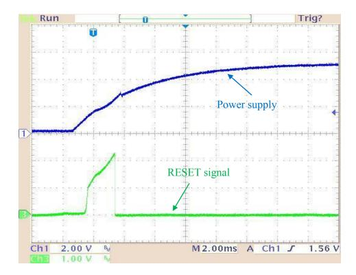
Figure 2.21 UVLO at Power-up transient
