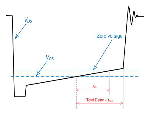
Figure 2.10  $V_{DS}$  waveform of the sync-FET for  $V_{OS} < 0$
