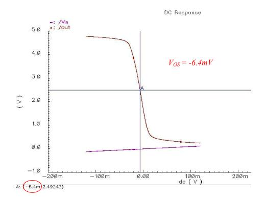
Figure 2.14 Voltage comparator offset voltage simulation
