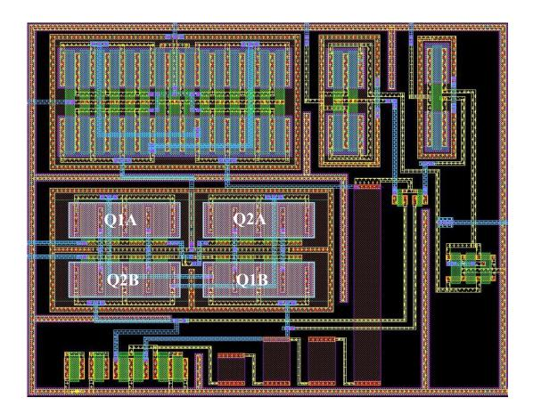
Figure 2.18 Layout of the voltage comparator
