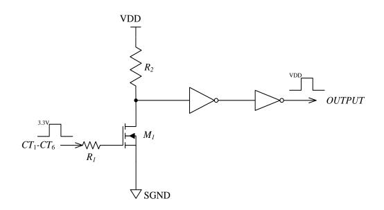
Figure 4.6 1<sup>st</sup> Level shifter
