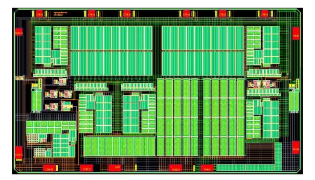
Figure 4.10 Layout of the CSD chip
