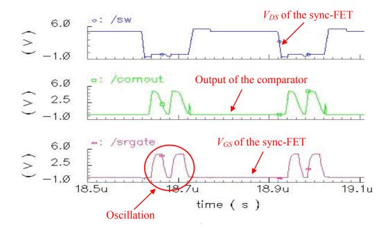
Figure 2.16 Simulation results for  $V_{OS} < 0$  without the ONE-SHOT control
