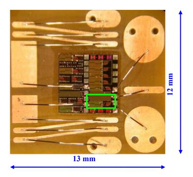
Figure 5.5 The buck PSiP before ferrite epoxy coating
