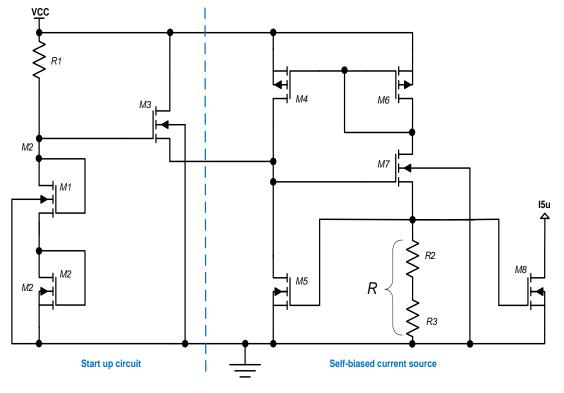
Figure 2.6 Current source circuit
