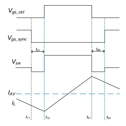
Figure 1.3 Switching waveforms of a typical synchronous buck converter
