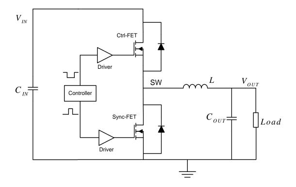
Figure 2.1 Conventional synchronous buck converter
