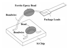
Figure 5.1 Concept of single bondwire with ferrite epoxy beads
