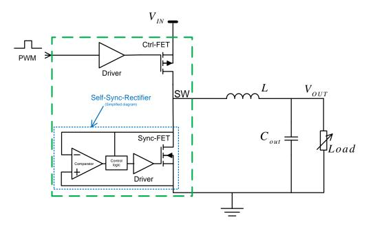
Figure 2.26 Simple buck converter testing circuit
