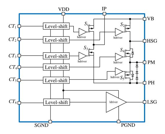
Figure 4.4 Simplified block diagram of the integrated gate driver
