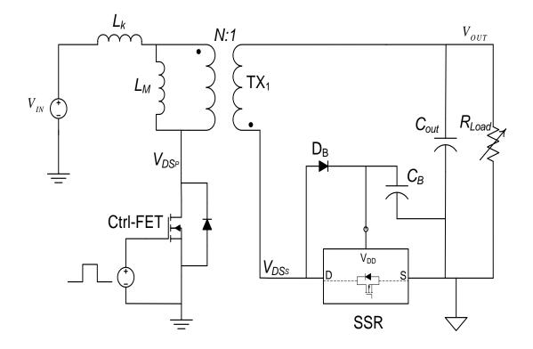
Figure 3.2 Circuit setup for simulations in Cadence
