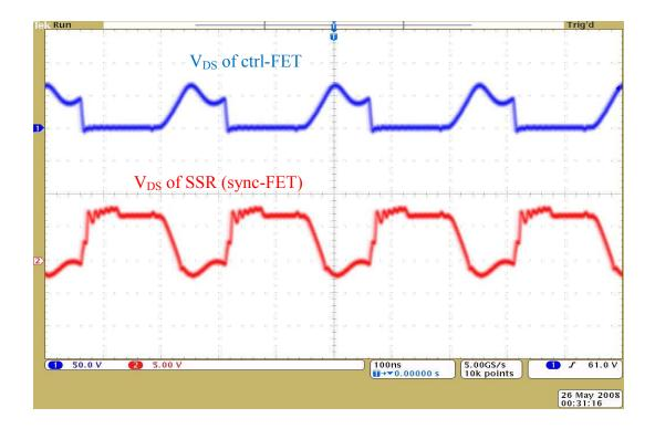
Figure 3.8 Operating waveforms at 4MHz
