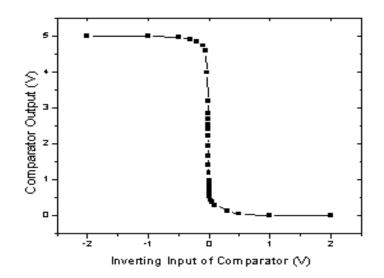
Figure 2.25 Comparator DC transfer characteristics
