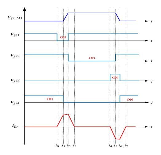
Figure 4.2 Waveforms of the CSD circuit
