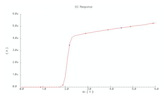
Figure 2.7 Current source power supply dependence (typ.)
