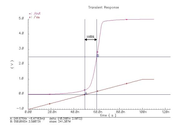
Figure 2.13 Propagation delay simulation for the voltage comparator (typ.)
