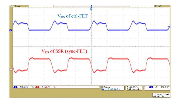
Figure 3.7 Operating waveforms at 2MHz
