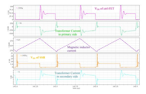
Figure 3.3 CCM Simulation
