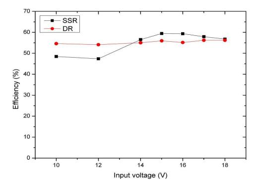
Figure 3.9 Measured efficiency vs. input voltage
