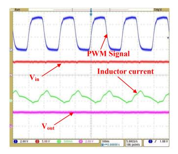
Figure 5.8 Operating waveforms of the PSiP with ferrite epoxy coating
