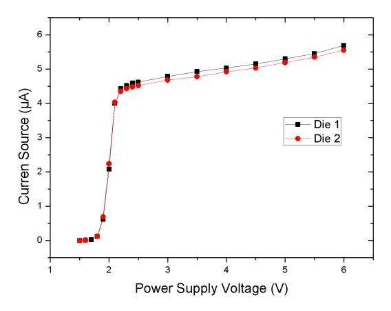
Figure 2.23 Current source testing results
