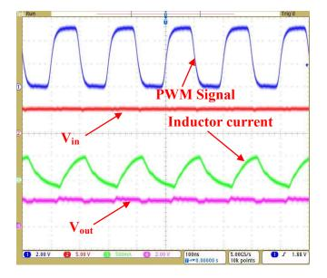
Figure 5.7 Operating waveforms of the PSiP without ferrite epoxy coating
