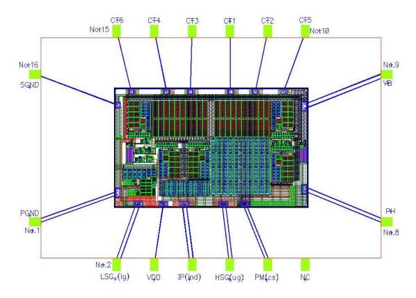
Figure 4.11 CSD chip bonding diagram
