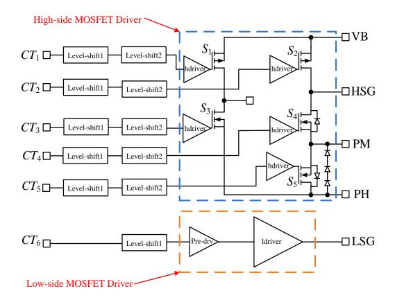
Figure 4.5 Schematic of the top level CSD chip
