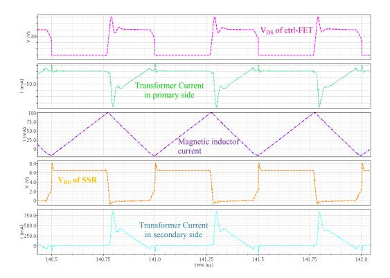
Figure 3.4 DCM Simulation results
