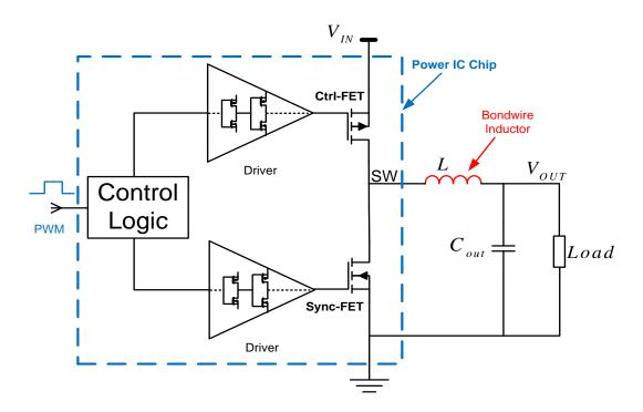
Figure 5.4 Schematic diagram of the buck PSiP
