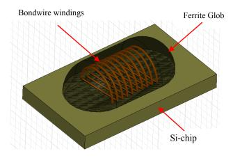
Figure 5.2 Concept of coupled on-chip multi-turn bondwire inductor
