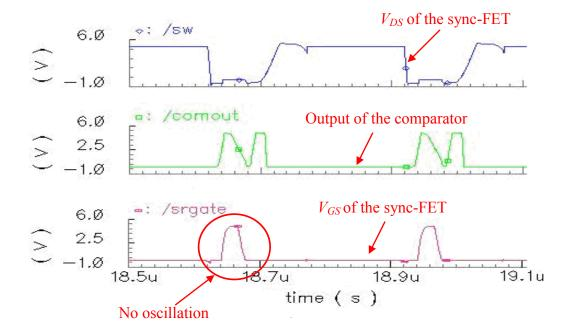
Figure 2.17 Simulation results for  $V_{OS} < 0$  with the ONE-SHOT control
