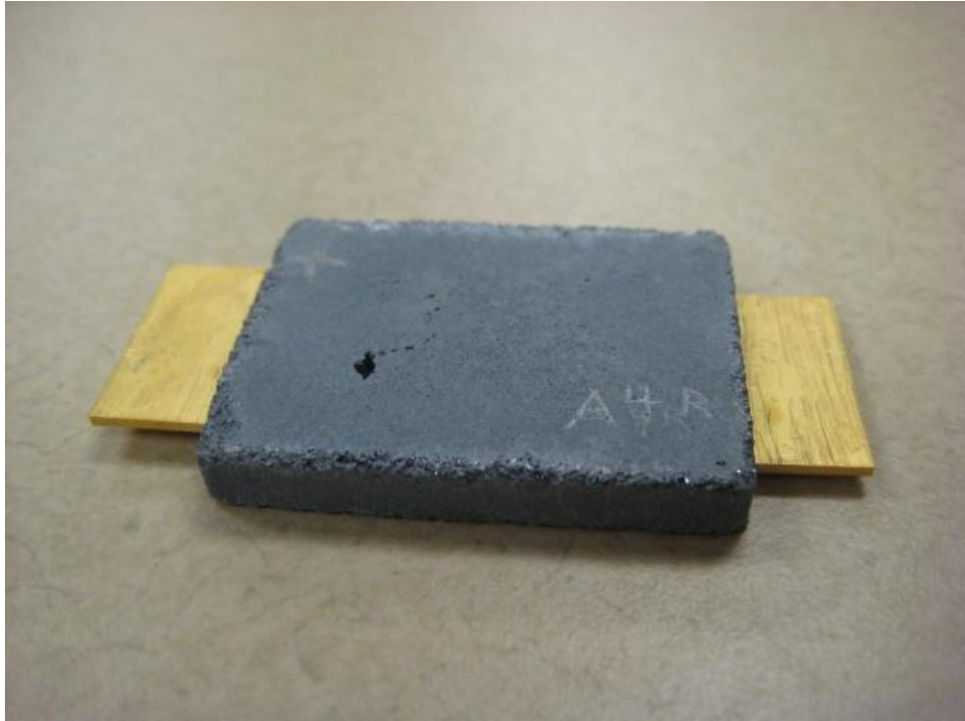
Figure 6.3 - Module A-4 with SiC Based Encapsulant
