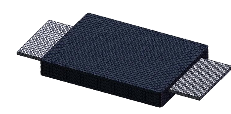
Figure 5.8 – Meshed View of Single Device Module Design
