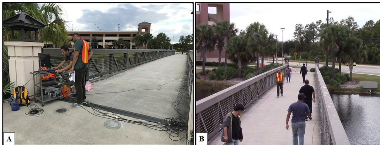
Figure 42 A: A perspective view from the footbridge and the data collection setup; B: The footbridge under the uncoordinated walking excitation of a group
