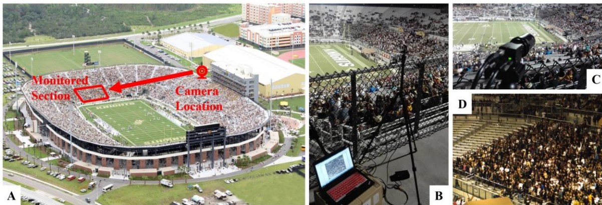
Figure 18 A: Overlook of the stadium showing the monitored section and the location of the camera; B: Experiment setup; C: The computer controlled industrial camera; D: One sample frame from the camera record
