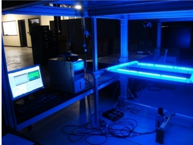
Figure 2.6: Picture of the TSP experimental setup in use; excitation and DAQ , the TSP is out of view at the top of the picture.
