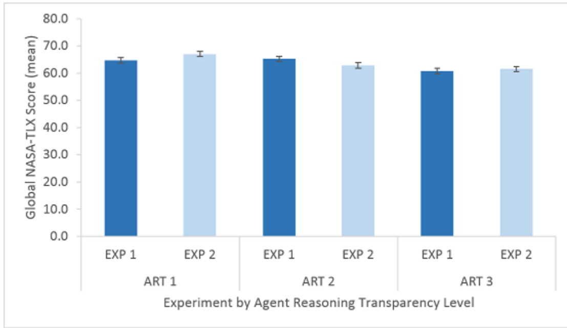
Figure 60. Average global NASA-TLX score, by experiment, for each agent reasoning transparency (ART) level. Bars denote SE.
