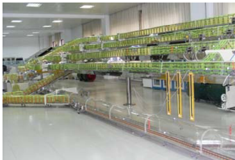
Fig.7: Cooling effect experiment equipment of common air cooler and bionic air cooler
