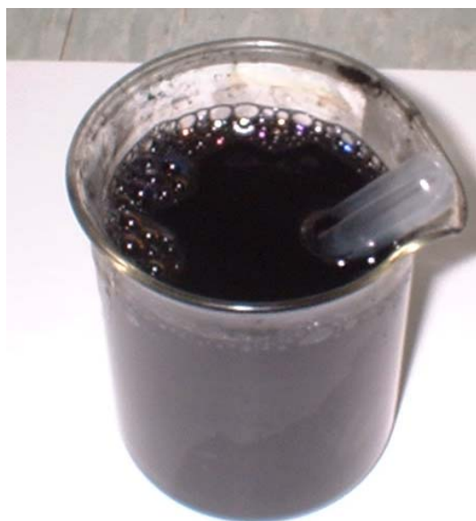
Figure 5.13: SWNT (1g/L) dispersed in copper bath with Pointe Scientific Inc Wetting Agent
