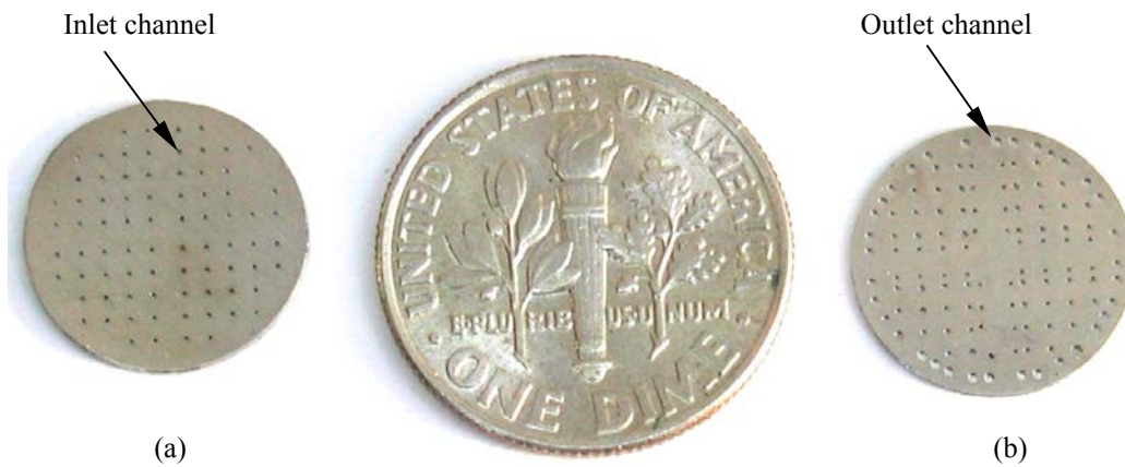
Figure 4.21: Finished nickel valve (a) Inlet (b) Outlet
