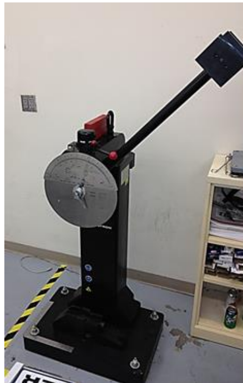
Figure 13. (a) Standard Type A Impact sample, and (b) Charpy Impact test fixture.
