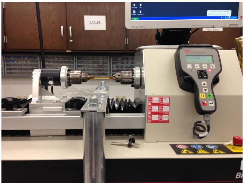
Figure 11. (a) Standard Torsion Specimen, and (b) testing fixture.
