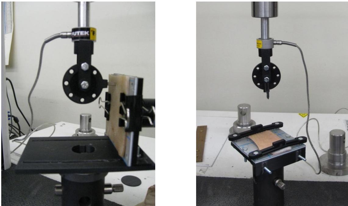
Figure 2.14: #15 Scalpel Slicing Test (left) #15 Scalpel Puncture Test (right)
