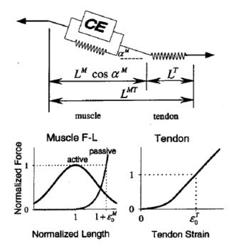
Figure 2.1 - Hill Muscle Model where L<sup>MT</sup> is muscle-tendon length, L<sup>M</sup> is muscle length, L<sup>T</sup> is tendon length, α<sup>M</sup> is pennation angle. Muscle and Tendon Force are normalized with respect to peak isometric force. Muscle length is normalized with respect to optimal fiber length. Tendon strain is defined as (tendon length – tendon slack length)/(tendon slack length). [12]
