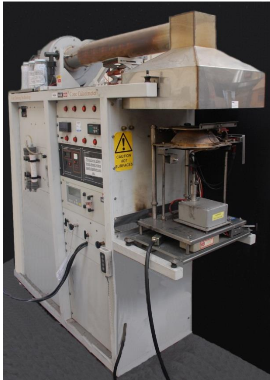
Figure 6: (a) Calorimetry Machine used for fire testing (b) Calorimetry Process Used for Heat Damage [Skovron, 2013]
