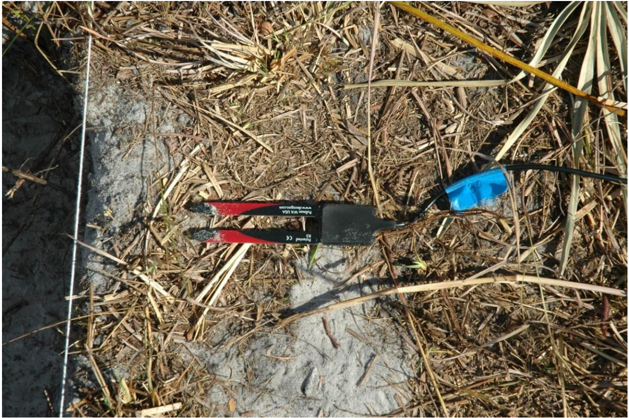
Figure 3: Soil moisture smart sensor prior to burial.
