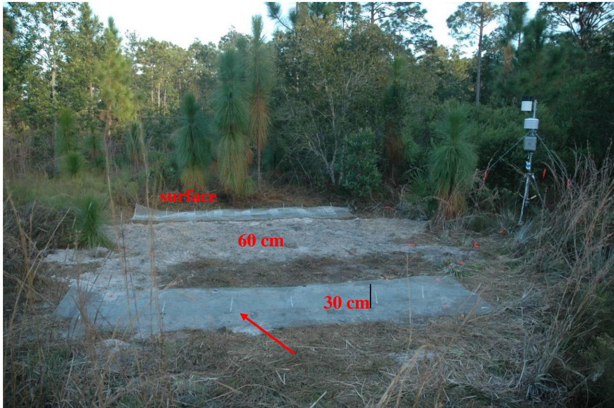
Figure 9: Shows the placement of the hardware cloth on the Ground Surface (top) and Trench 1 (bottom), and the exclusion of it on Trench 2 (middle). Zip ties are indicated by the red arrow.
