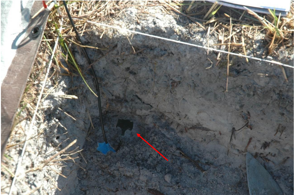
Figure 4: Soil moisture smart sensor with probe placed horizontally into the bottom of the trench.
