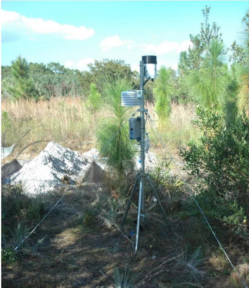
Figure 2: HOBO weather station at the research site includes a temperature smart sensor, a rain gauge smart sensor, and three soil moisture smart sensors.
