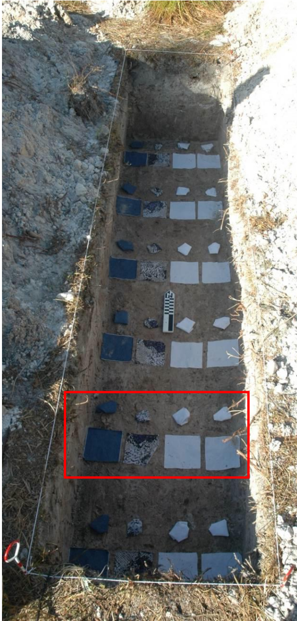
Figure 6: Trench 2 (60 cm) showing the layout of fabric swatches and distance between each group and edge of pit. For example, one month of samples is marked by the red box.
