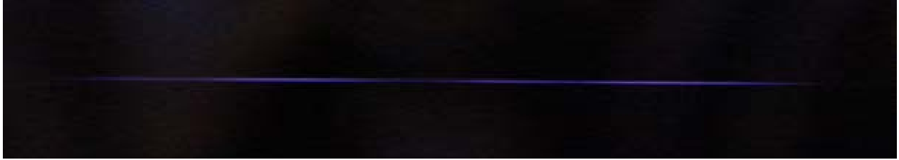
Figure 32: Nitrogen fluorescence obtained when a telescope with a 40 cm equivalent focal length was used in conjunction with the helical beam synthesizer. Two longitudinally separate ionization peaks can clearly be observed.
