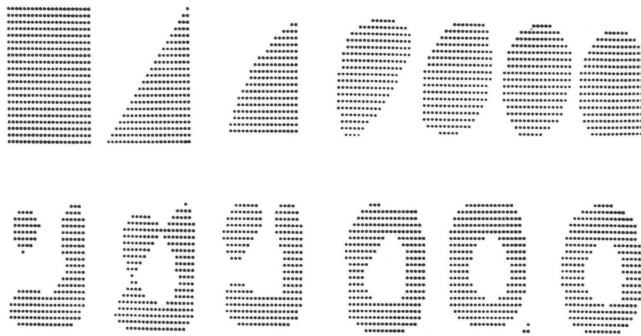
Fig. 15. Two-dimensional MoM reconstruction of the letter O. First row (left to right): reconstructions using the zeroth through sixth moments. Second row: seventh through twelfth.
