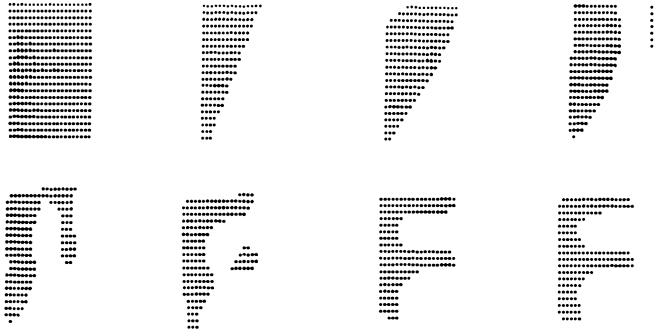
Fig. 11. Two-dimensional MEP reconstruction of the letter F. First row (left to right): reconstructions using zeroth through third moments. Second row: fourth through seventh.
