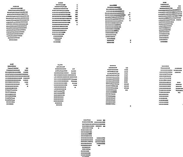
Fig. 12. Two-dimensional MoM reconstruction of the letter F. First row (left to right): reconstructions using zeroth through third moments. Second row: fourth through seventh. Third row: eighth through eleventh. Fourth row: twelfth.
