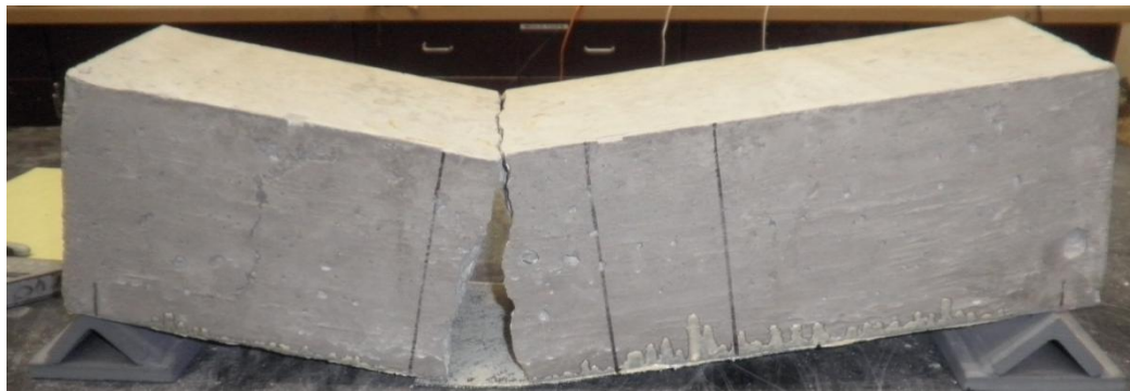
(a) Specimen at Failure
