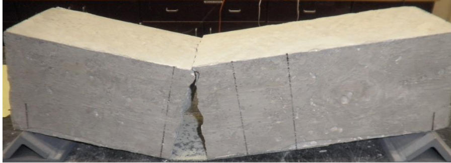
(a) Specimen at Failure
