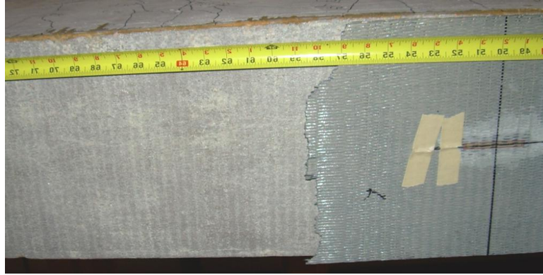
Figure 107. PU Baseline CFRP Rupture Plane
