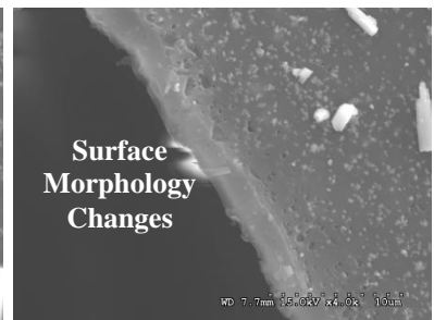
Figure 66. 60 Day Seawater Void Wall
