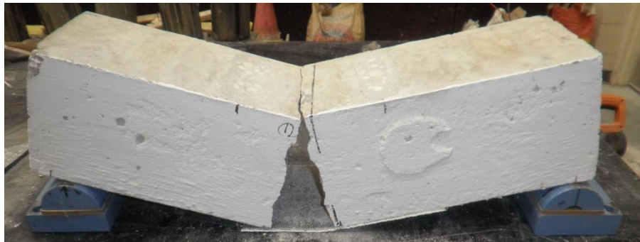
(a) Specimen at Failure
