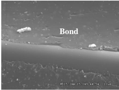
Figure 74. Fiber After Beam Failure – 30 Day
