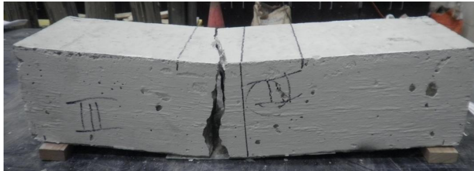
(a) Specimen at Failure
