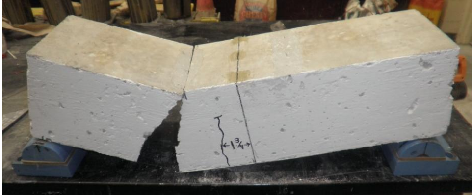
(a) Specimen at Failure
