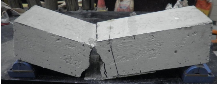
(a) Specimen at Failure
