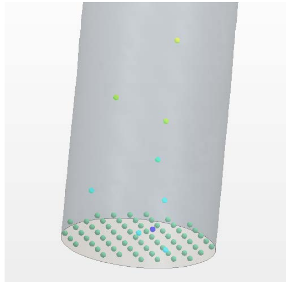
Figure 17 - Particle injection at LVAD inlet.
